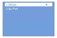
Output shift includes two selections: "Whole" and "By Port". In the setting interface of "Whole", you can rotate the knob to set X and Y of the whole image, then save it; in the setting interface of "By Port", you can set X and Y of the image of each net port respectively and also save it.
