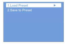
In the submenu, 16 preset parameters can be saved, and every preset parameter includes all parameter information of the video source setting (scaling, cropping, several layers display, EDID, etc.). Users can also directly load the saved preset parameters to display the image according to their needs so that they don't need to set up all the parameters again.
