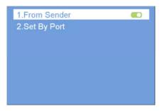
In the submenu, press the knob/OK to set sender as the connection source. At this time, rotate the knob and press the knob/OK to enter the setting interface, select the net port of what needs to be set, then set the offset values of X and Y. You can also set the tile width, tile height, row count, column count and link type of the corresponding cabinets. Save all of the parameters afterwards.
